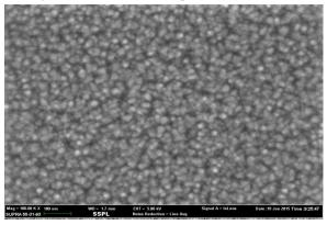
**Fig: 5(b).** SEM micrographs of CdTe at 100KX magnification with 5KV at deposition rate of 1 Å/sec
