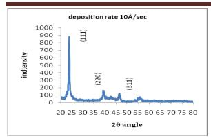
**Fig: 3(c).** CdTe deposition on Si at deposition rate of 10Å/sec
