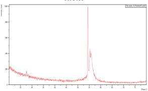
Fig: 3(d). XRD Analysis of Polished Silicon
